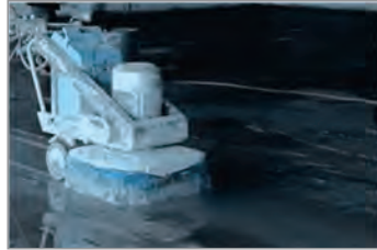
Floor grinding equipment
